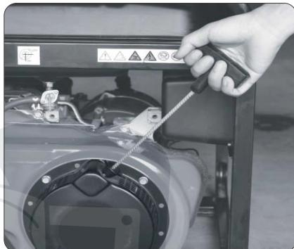
(e) After the engine started, return the choke lever gradually to "OPEN" position.
